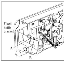
Note: To adjust, loosen two thread trimmer cam clamp screws A.
