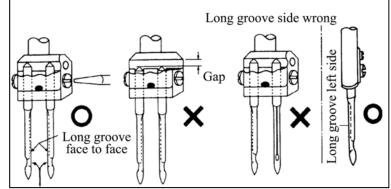
up into the needle bar(or needle clamp) as deeply as it will go, with the long groove of the needle faced left side(ro face to face). Tighten the needle set screw securely.
