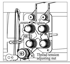
To adjust needle thread tension, turn each tension adjusting nut.
