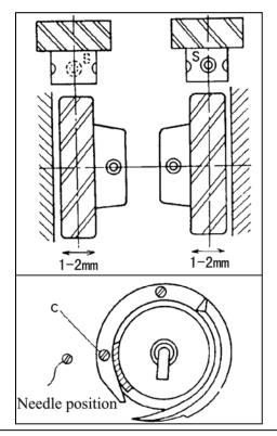
(3) Approximate position of hook "C"screw of hook should be found close to the needle when the needle is at DOWN position.
