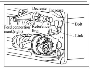
When fabric with large elasticity is sewn, or when thickness of fabric changes, the vertical stroke (movable range) of the presser feet should be adjusted as follows:
