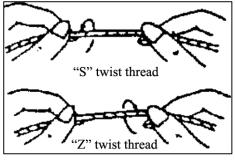
right needle. When discriminate use "Z"twist thread in both the needles. For bobbin thread, "S"twist thread as well as "Z"twist thread can be used.
